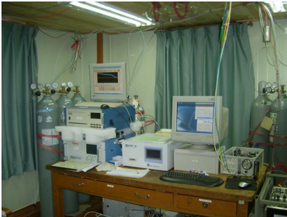
CO 2 concentration measurements based on NDIR
