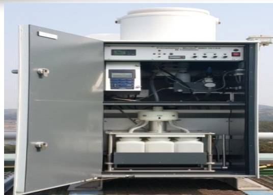
Automatic Dry & Wet Sampler - wet (at precipitation), dry (monthly)
