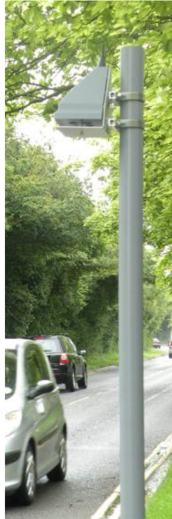
Fig. 11. Static sensor unit (or node) plus mounting baseplate. CO, NO, NO 2 , temperature and relative humidity are recorded, along with GPS location and time. A view of the open sensor node is also shown (left).
