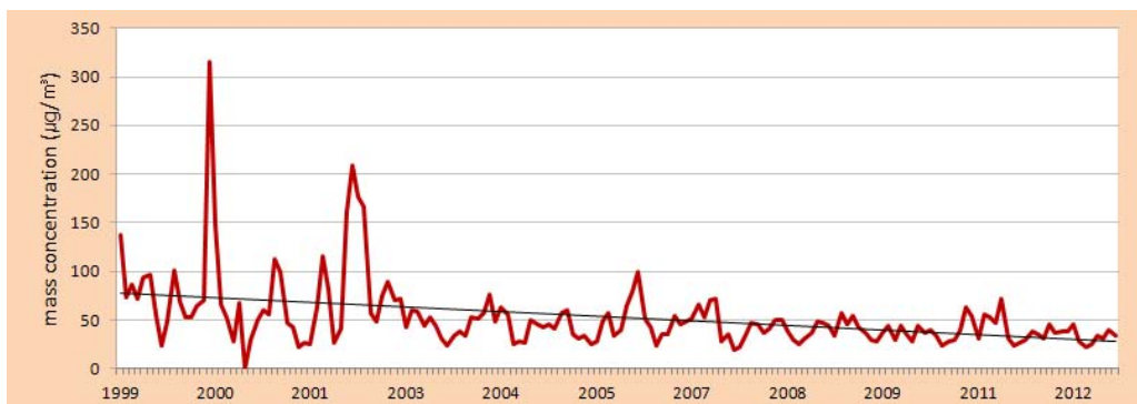
Fig. 4. Monthly mean time series of mass concentration observed by \beta -ray \text{PM}_{10} in the KGAWC from 1999 to 2012. Black line indicates the linear regression for mass concentration in ambient air over the Korean Peninsula.
