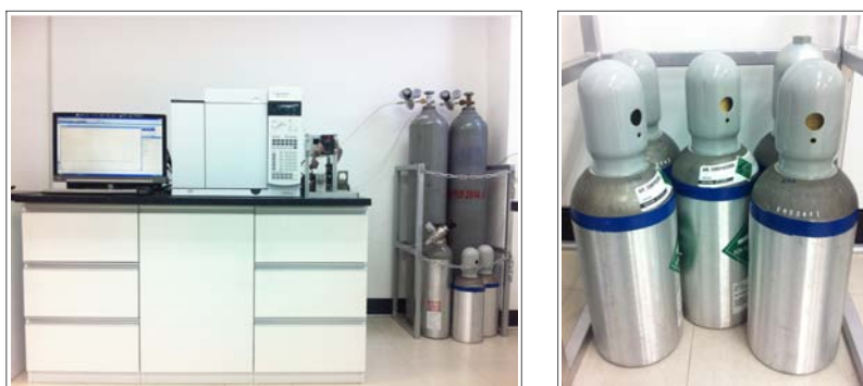
Figure 4. Analytical system (left) and primary standard gases (right) to prepare laboratory and transfer standards traceable to the WMO SF 6 mole fraction scale
